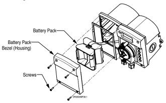
Figure 7. Inserting D-Cell Batteries
