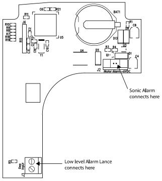
Figure 7a. Low-Level Alarm Connections
